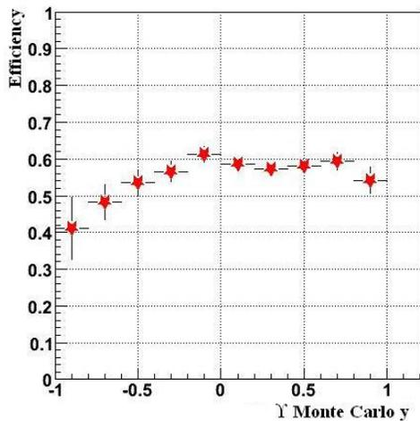
Figure 4. Embedded TPC tracking efficiency versus Monte Carlo  $\Upsilon$  rapidity.
