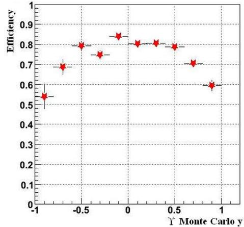
**Figure 2.** Embedded L2 Efficiency calculation versus the Monte Carlo  $\Upsilon$  rapidity for the 2005 STAR geometry. In 2005 the complete STAR BEMC was not available. The negative  $\eta$  and negative  $\phi$  quadrant was missing.
