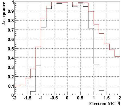
**Figure 1.**  $\eta$  distribution of the acceptance for Monte Carlo generated electrons. The red curve represents those with a single hit in the BEMC, the black curve represents those that left at least 0.25 GeV in the BEMC.
