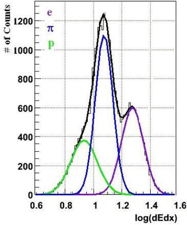
**Figure 7. Gaussian fit for the momentum range  $4 < p < 6$  GeV/c. The  $\chi^2/\text{dof}$  is 205.3/111 for this particular range. The fit is improved when smaller momentum slices are used.**
