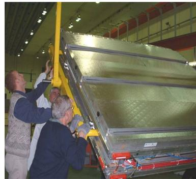
**Figure 4.** RPC mounted on a DT chamber.
