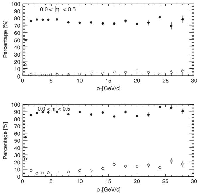
Fig. 3. Reconstruction efficiency (full symbols) and fake rate (open symbols) as a function of transverse momentum in the barrel region of the tracker for central Pb + Pb collisions with  $dN/dy \approx 3000$ . Upper: track quality cuts optimized for low fake rate (number of hits  $> 12$ , fit probability  $> 0.01$  and  $dca < 3$ ). Lower: track quality cuts optimized for high efficiency (number of hits  $> 12$ ).
