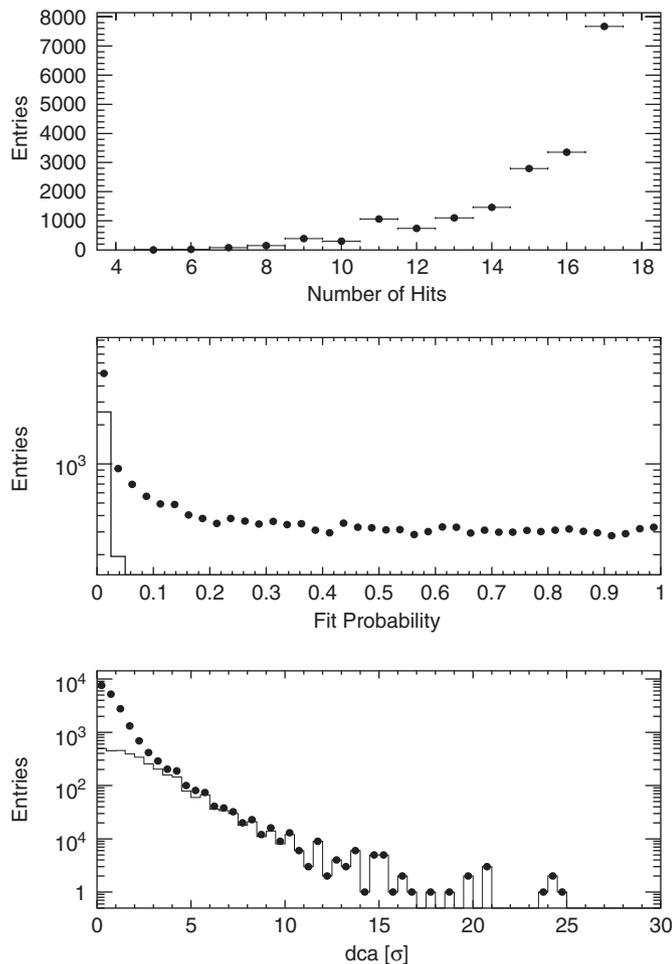
Fig. 2. Track quality measures for all reconstructed tracks (symbols) and for fake tracks contained in the sample (histogram). Upper: number of hits per reconstructed track. Hits on stereo layers are counted as two separate hits. Center:  $\chi^2$  probability distribution for reconstructed tracks. Lower: distance of closest approach, dca, to the primary vertex normalized by the error.
