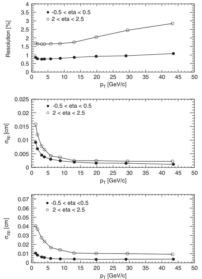
Fig. 4. The  $p_T$  dependence of the track parameter resolution achieved in heavy ion events in the barrel region (full symbols) and in the forward region (open symbols). Upper: transverse momentum resolution. Center: transverse impact parameter resolution. Lower: longitudinal impact parameter resolution.
