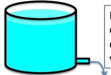
Electrical *Capacitance* is similar to the cross sectional area of a fluid reservoir or standpipe. Electrical charge corresponds to amount (volume) of the stored fluid. And voltage corresponds to the height of the fluid column.
