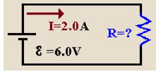
Solution:  $V = IR \Rightarrow R = V/I = 6.0 V/2.0 A = 3.0 \Omega$
