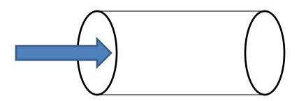
R = (Fluid properties) x (geometric properties) =  $(8\eta/r^2)$  x (L/A) =  $8\eta L/(\pi r^4)$
