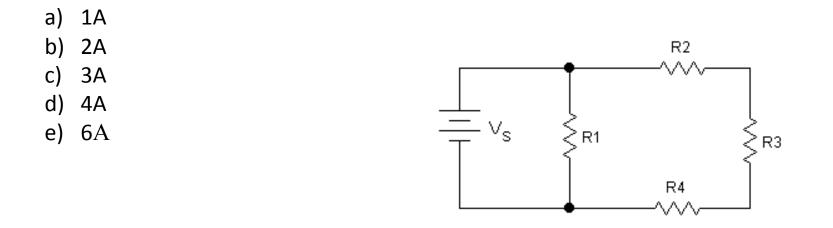
Solution: R2 + R3 + R4 = 6 $\Omega$ . Two parallel 6 $\Omega$  resistors have an equivalent resistance of 3 $\Omega$ . The current through the battery we get from Ohm's law,  $I = V/R = 12V/3\Omega = 4A$
