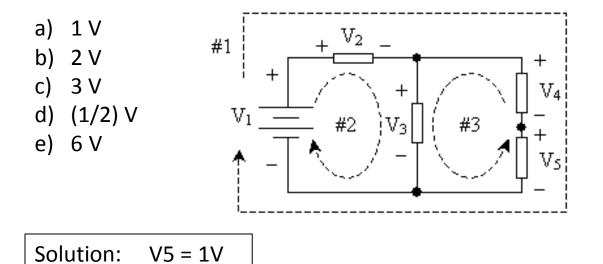
Mesh #1:  $-V_1 + V_2 + V_4 + V_5 = 0$ Mesh #2:  $-V_1 + V_2 + V_3 = 0$ Mesh #3:  $V_3 - V_5 - V_4 = 0$
