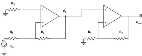
Figure 1: Schematic diagram for a two-stage amplifier.
