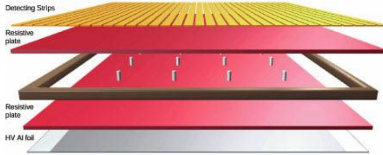
Figure 3.23: Design and layers of a single Resistive Plate Chamber single gap [41].
