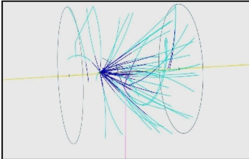
Figure 2: (Color Online) Fixed target collision as seen by the STAR detector and reconstructed. Note that the vertex is displaced from the beam line (the yellow line) and also displaced from the center of the detector (denoted by the pink line). All of the tracks are to one side of the vertex (to the right) rather than being symmetric about the collision point.
