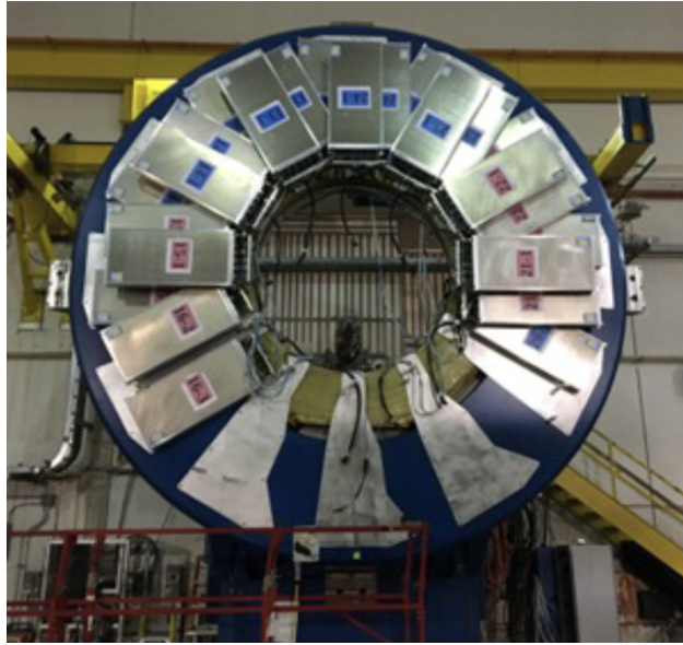
Figure 2.5: Endcap time-of-flight detector prior to installation. Photograph courtesy of Daniel Cebra.
