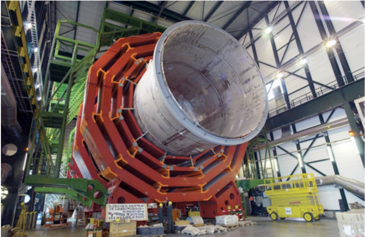
Figure 3.7: The CMS solenoid magnet in gray is shown being inserted into CMS. The iron return yoke which holds the barrel muon chambers, is shown in red [56].
