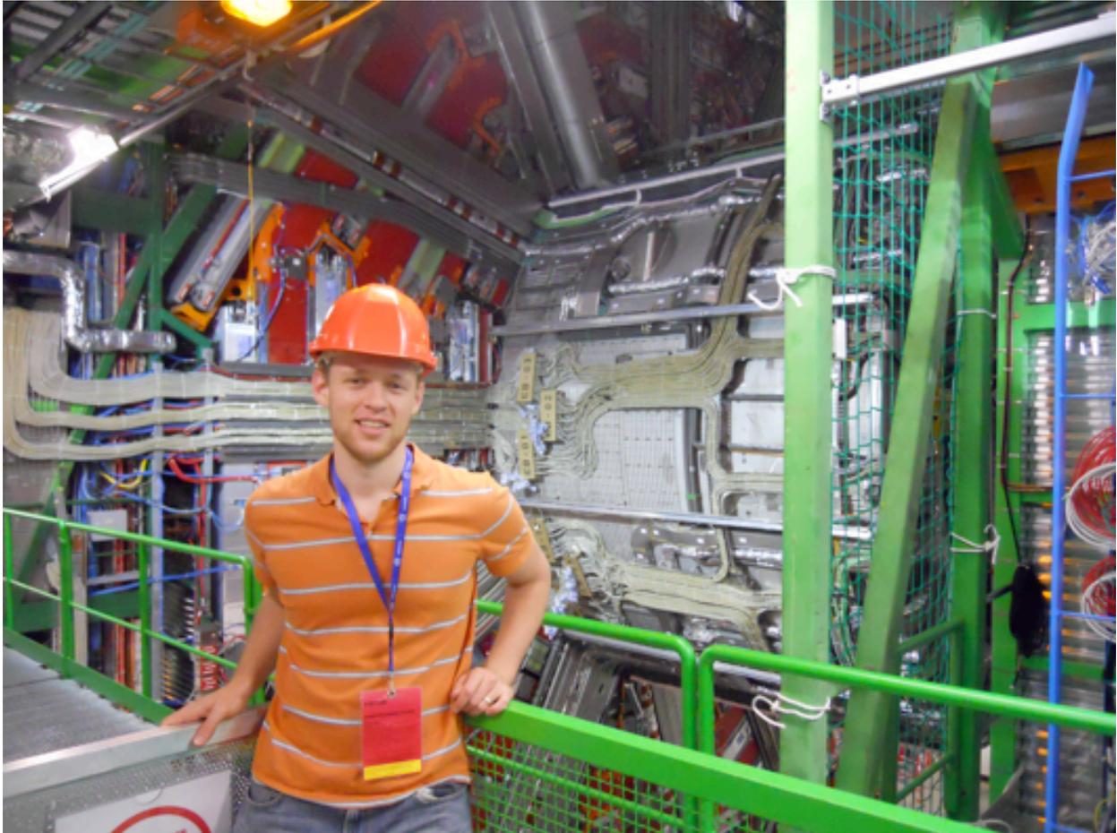
Figure 3.8: During Long Shutdown 1 (February 2013 - November 2015), the LHC and the detectors underwent significant repairs. During this time, I was allowed to go down into the viewing area of the detector to see CMS pulled apart, with a good view of the return yoke (in red), the magnet (in silver) and all of the cabling [60].
