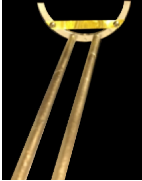
Figure 3.1: Photograph of the STAR fixed target with accompanying support structure.
