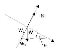
What we need to do is solve for the acceleration. With the acceleration we can use one of the kinematic equations to solve for the velocity.  $(F_{net})_x = ma_x$ =  $W_x$  =  $Wsin\theta$  =  $mqsin\theta$  =  $ma_x$  $a_x = gsin\theta = (9.8m/s^2)(sin10^\circ) = 1.7m/s^2$
