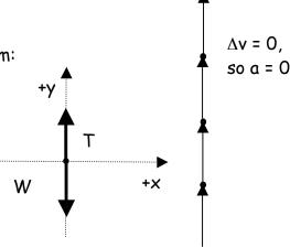
$(F_{net})_y = ma_y$ since v is not changing  $a_y = 0$ T-W = ma\_y = 0 T = W = mg = (1000kg)(9.8m/s<sup>2</sup>) = 9800N
