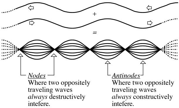
Properties of the two waves that are superposed to make a standing wave:
